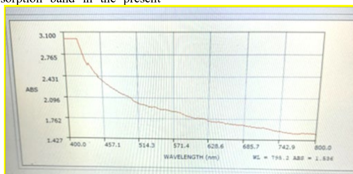
Fig. 3. UV-VIS spectroscopy for silver nanoparticles synthesised using Aegle marmelos leaf extract.
